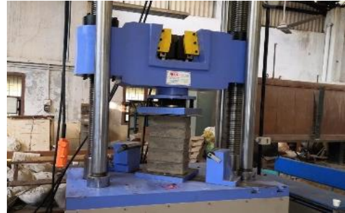
Figure 2. Prism Specimen Tested
