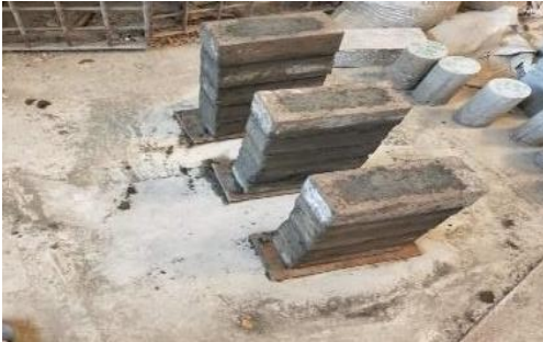
Figure 1. Prism Specimen Casted
