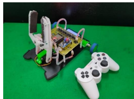
Figure 7. Shape Transporter Robots and controllers dual shock 3
