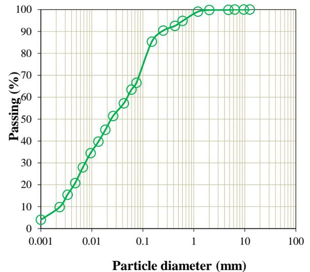
**Figure 1.** Particle size distribution curve of soil
