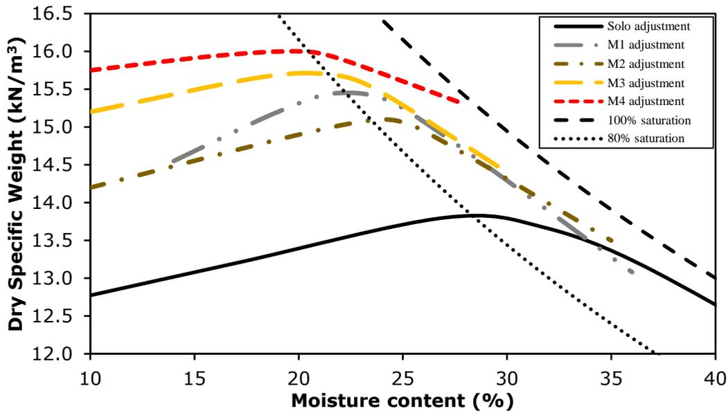
**Figure 3.** Clay compaction curves
