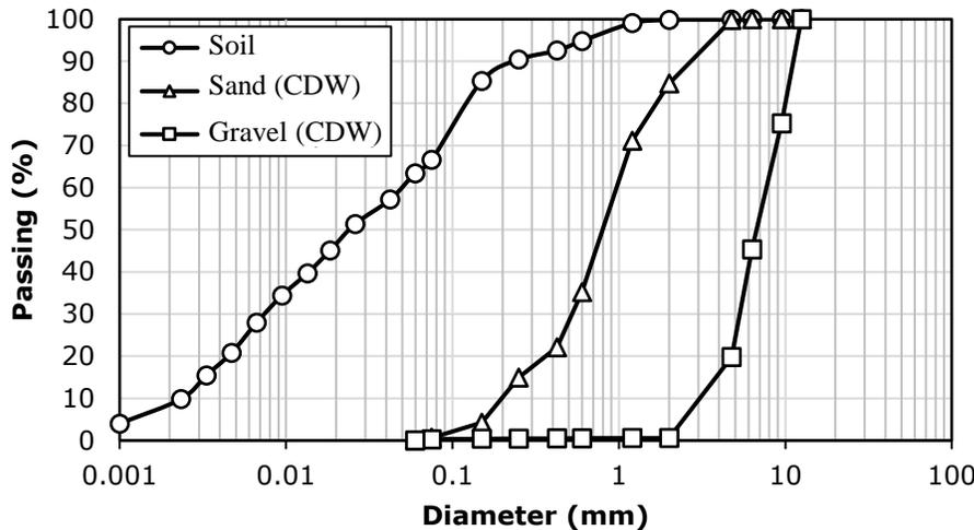
**Figure 2.** Particle size distribution curve of CDW
