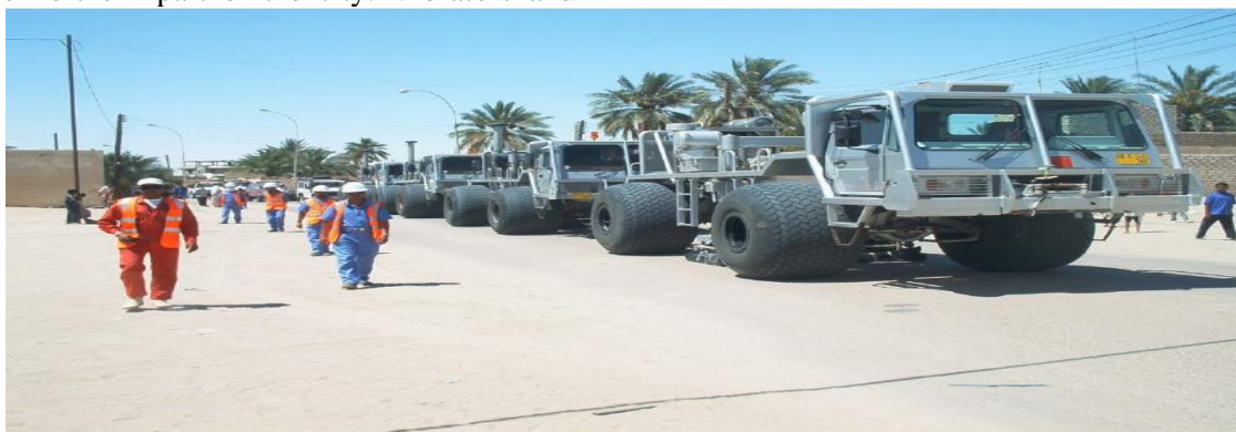
Figure 5. The seismic acquisition operation in Jakhira City uses seismic trucks.
