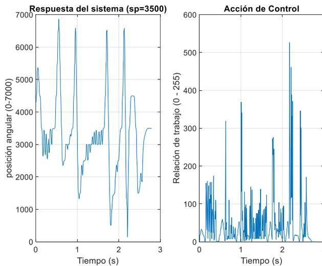
Figure 20. Response and control action of the PD2DOF regulator.
