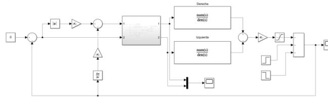
Figure 7. PD control applied to the two-wheel system.
