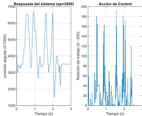
Figure 18. Response and control action of the PD regulator.
