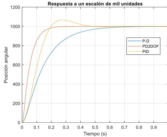
Figure 14. Response curves of the different control techniques.
