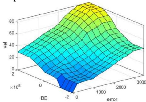
Figure 12. Blurred PD controller control surface.
