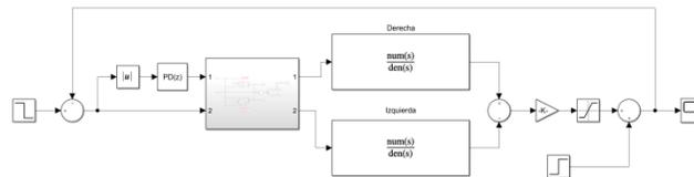
Figure 6. PD control applied to the two-wheel system.
