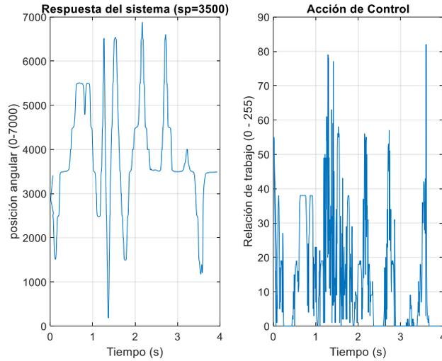
Figure 19. Response and control action of the PI-D regulator.
