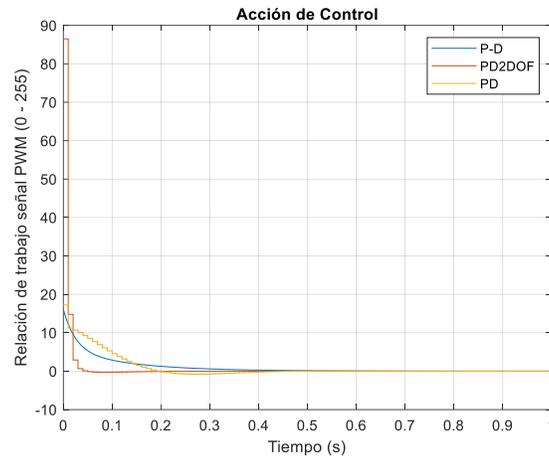
Figure 15. Response curves of the different control techniques.
