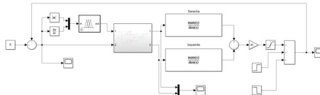
Figure 13. Fuzzy PD control applied to the two-wheel system.
