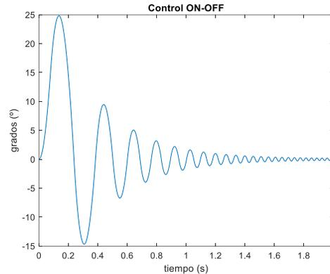
Figure 5. System response with an ON-OFF control.
