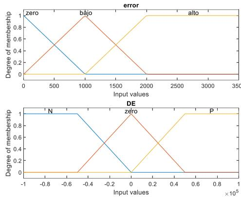
Figure 10. Fuzzy sets and linguistic labels of the variables: error and error derivative.
