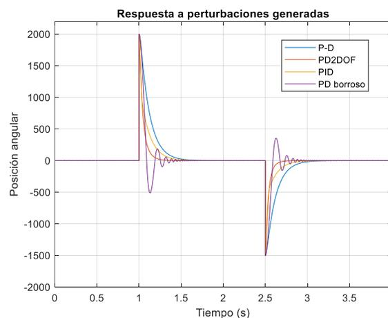
Figure 16. Response of controllers to disturbances.
