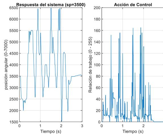
Figure 21. Response and control action of the fuzzy PD regulator
