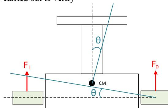
Figure1. Line follower robot free body diagram.
