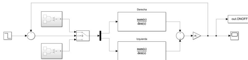
Figure 4. Line follower robot model, ON-OFF control.
